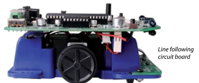
Line following circuit board Plastic chassis with battery compartment, motors with gear boxes and 2 wheels
