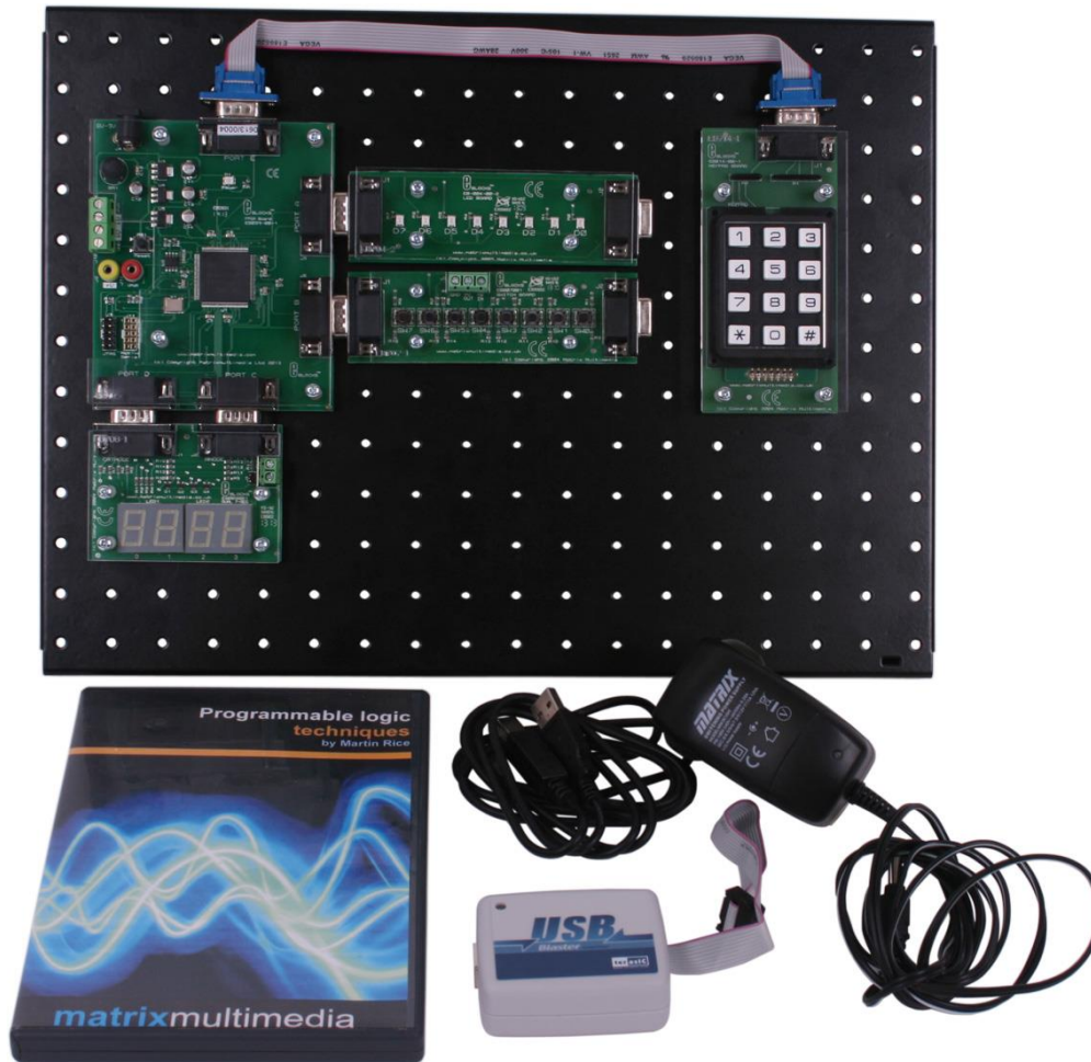
Fig 1.1: E-blocks FPGA Solution
