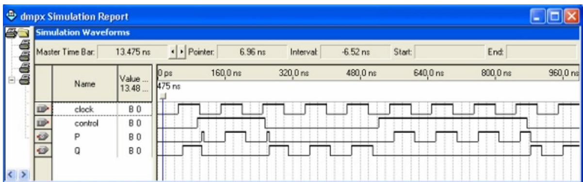
Fig. 7.2: Simulation result for two_way_dmpx design.
