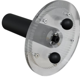
Tapped cylinder attached to circular protractor (Worksheet 2)
