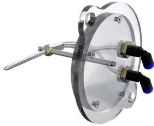
Pitot-static tube experiment holder (Worksheet 1)
