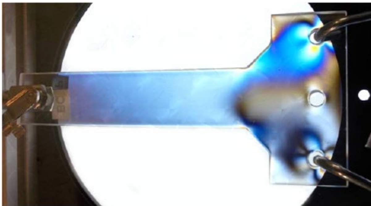
Welded Seams at 200N
